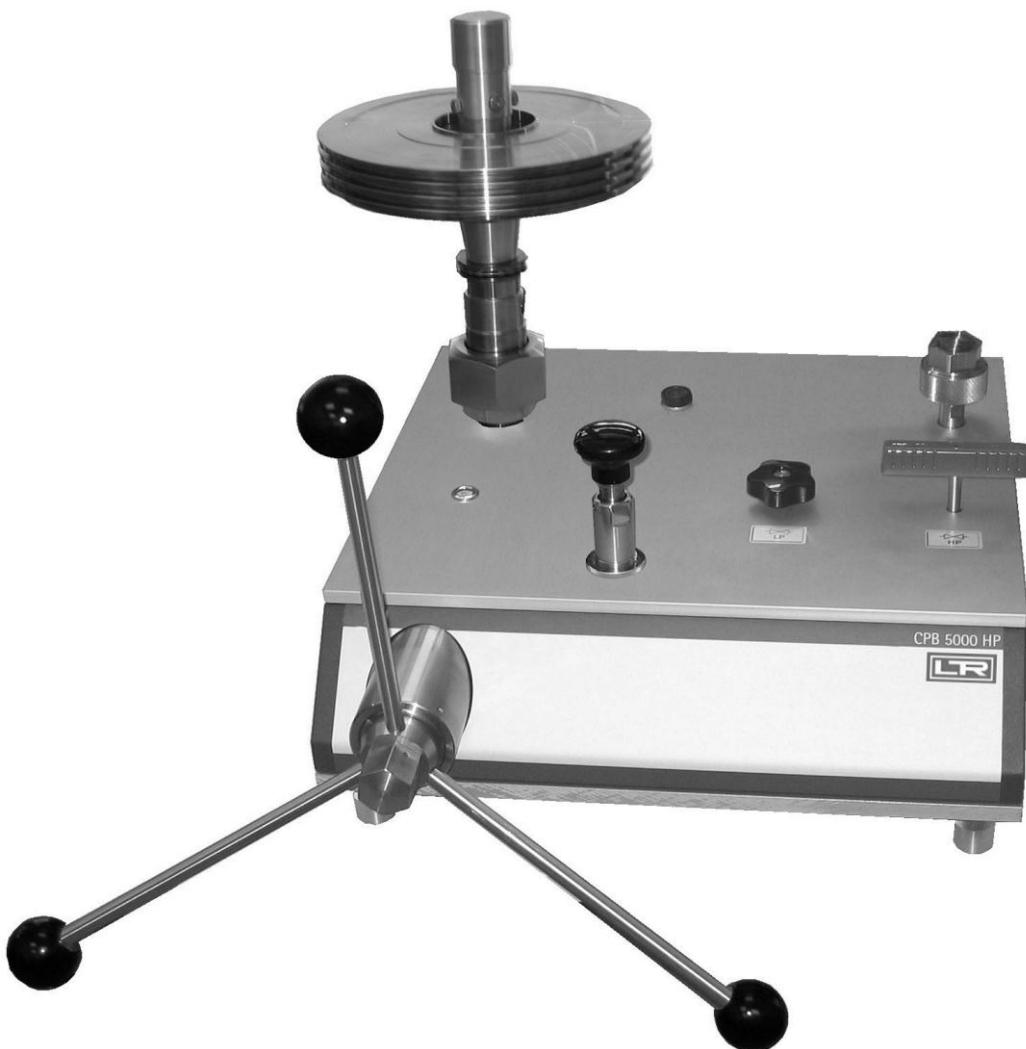
Deadweight Tester / Pressure Balance High-Pressure LR-Cal / CPB 5000-HP
