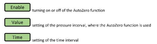
AutoZero function serves for elimination of undesirable instability at displaying the zero value of the manometer. For correct AutoZero function it is necessary to set also the menu items Value and Time.
